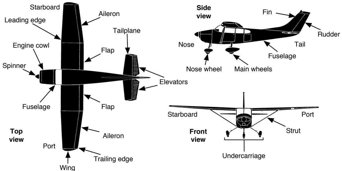
The primary flight controls on any powered aeroplane are: elevator (pitch), aileron (roll), rudder (yaw) & throttle. Gliders have no engine or throttle but their controls are otherwise the same.
