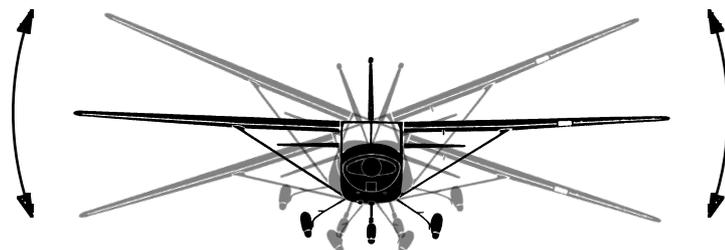
the operation of the ailerons. To roll left, the left aileron is raised and the right aileron lowered. The combined effects of the airflow on the controls lowers the left wing and lifts the right wing. The operation is reversed to roll right.
