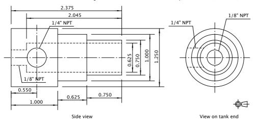
Item C: 2-Hole tank fitting. Material: Aluminium 2011 T6. 1 required: Vent (starboard upper rear)
