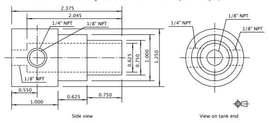
Item B: 2-Hole tank fitting. Material: Aluminium 2011 T6. 1 required: Reserve (starboard)
